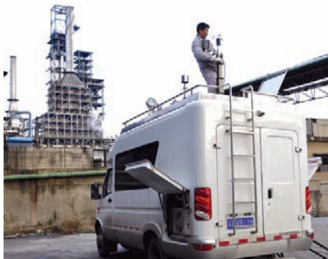
On-Line monitoring system for discharged pollutants
