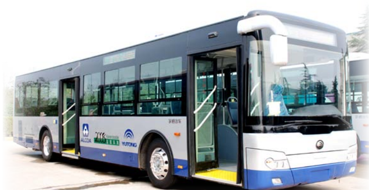
Environmental friendly aluminum – intensive bus by Alcoa and Yutong Bus
