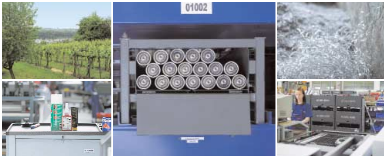
A specially developed container has eliminated the need for an outer packaging for the delivered folding rollers.
