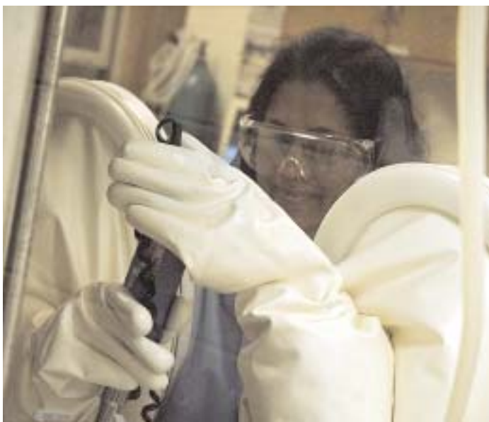
The use of isolators provides a controlled, sterile work environment that is less energy intensive than traditional manufacturing environments. Baxter has integrated the use of isolators into many of its facilities, including Round Lake, Illinois, United States.
