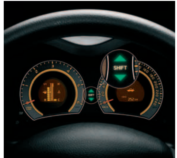
Gear Shift Indicator in the Toyota Auris
